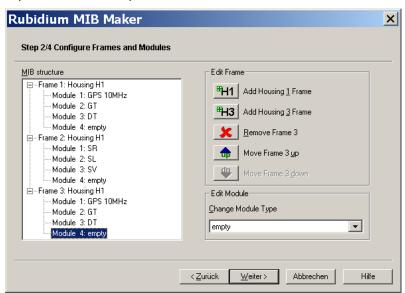
The "MIB structure" window indicates the current built system. Add or remove RUB frames pressing the buttons of "Edit Frame". Clicking on a module at the MIB structure enables you to select the type of the module out of the "Edit Module" dropdown list.
