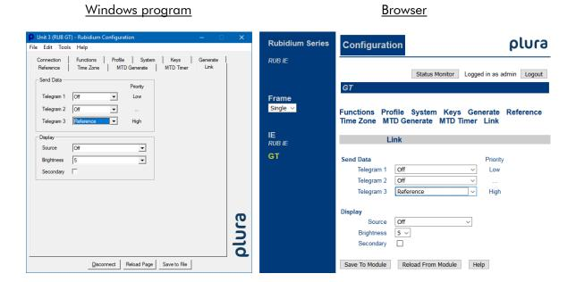
Within the "Link" submenu, set <u>one</u> of the three possible telegrams to "Reference". The NTP Server automatically detects the telegram and synchronizes its clock.
