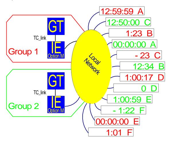
Each Ethernet module offers NTP Server functionality. Therefore, NTP Clients can access the one or the other NTP Server.
