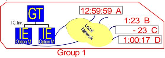
Even if there are two MTD central units for redundancy (two RUB GT modules + RUB SL as changeover unit), there will be <u>one</u> MTDoE group only. Both RUB GT modules have to receive the same set-up. Both RUB GT modules have to be connected to the RUB SL module. All modules have to be connected to the same  $TC\_link$  interface.
