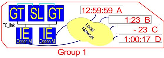
The NTP Server at each Ethernet module will be available always, regardless whether an Ethernet module is active or inactive regarding MTDoE operation. This applies to both installations shown in the examples above. Therefore, NTP Clients can access the one or the other NTP Server.
