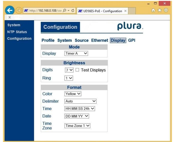
The configuration of the display, the selection of available display formats, brightness and colors are done via the USB interface or via a standard internet browser (Ethernet displays only). Software updates are made using the standard USB interface.
