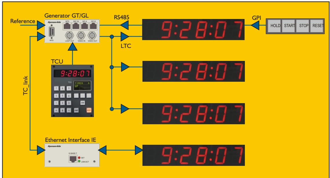
There are several included serial protocol decoders available for the input data communicated via serial interface. Protocols are selected in the configuration mode of the display. An Plura specially developed MTD protocol mode is also included. MTD is a studiotimer solution developed and designed by Plura to deliver several information like countdown timers, difference timers, or timezones.
