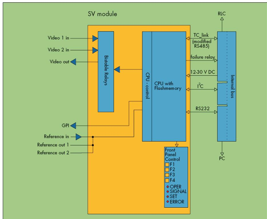
LEDs located on the front of the module indicate the operating status. Built-in GPIs can be programmed to signal errors or other pre-programmed warnings. The backlit keys on the front of the module can be programmed to suit the user specific needs (e.g. a key could be programmed to manually switch incoming sources).
