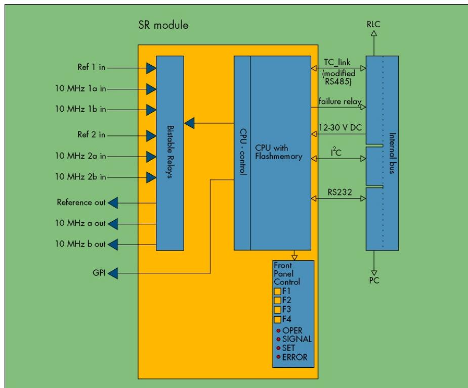
LEDs located on the front of the module indicate the operating status. Built-in GPIOs can be programmed to signal errors or other pre-programmed warnings. The backlit keys on the front of the module can be programmed to suit the user specific needs (e.g. a key could be programmed to manually switch incoming reference sources).
