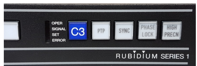
RUBIDIUM H1 C3 module in H1 housing
