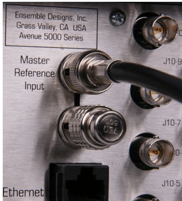
Connecting a Timing Reference to the Master Reference Input on the rear of the Avenue Frame. The loop through is terminated with a 75 ohm termination.
