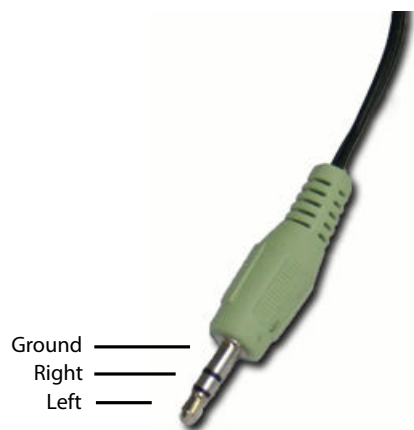
Example of a 1/8 inch mini-jack audio cable
