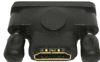
Example of a DVI-to-HDMI adaptor, HDMI end
