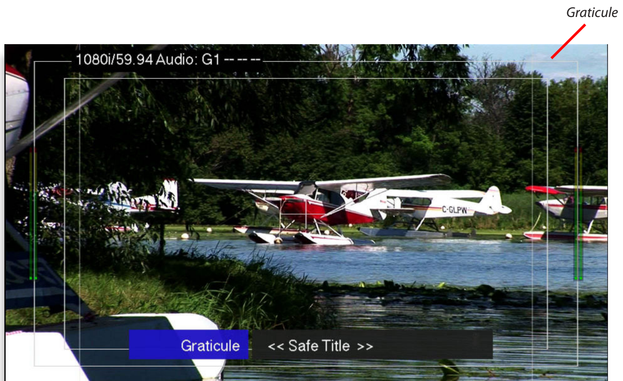
Example of on-screen display while adjusting the Graticule control from the front panel
