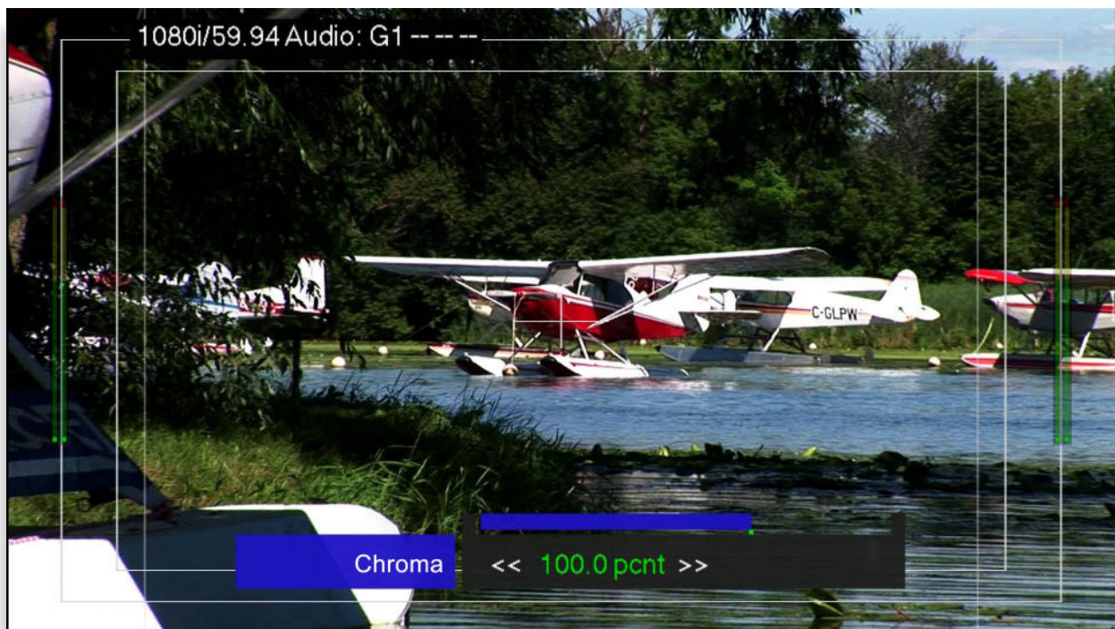
Example of on-screen display while adjusting the Chroma control from the front panel
