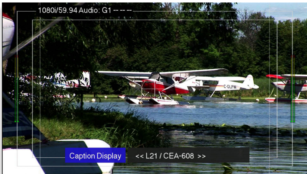
Example of on-screen display while adjusting the Caption Display control from the front panel
