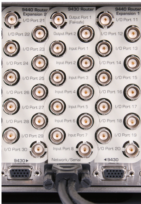
Rear BNC connectors and the HD-15 connector on the 9430
