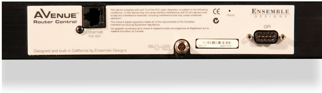
The rear of the Router Control Panel. Note the three connectors: the RJ-45 Port, the Power Input, and the 9-Pin GPI Connector.
