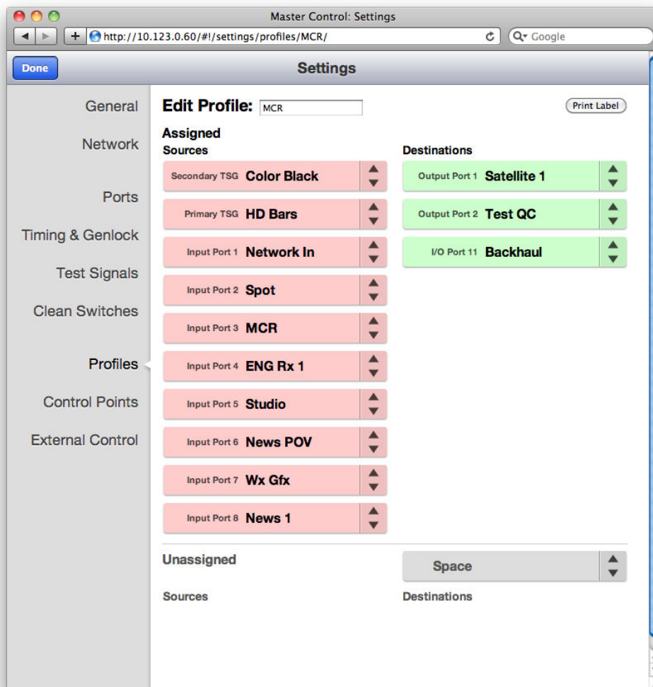
An example of a Master Control Room (MCR) Profile with 10 Sources and 3 Destinations
