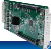
The 9550 HD Processing Frame Sync accepts a 3 Gb/s or 1.5 Gb/s high definition video or standard definition video signal for processing, synchronization and timing.
