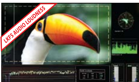
LKFS Audio Loudness Measurement - Digital Loudness Audio Metering with selected channel measurement in LKFS scale.
