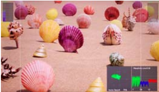
Display Advanced Waveform & Vector Scope simultaneously with line select
