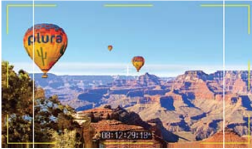
Various and User defined Markers Display, Safe area in HD and SD.
