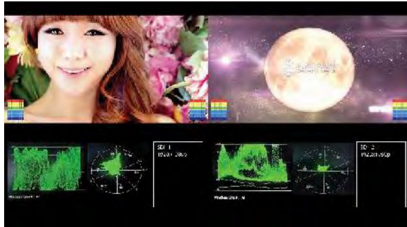
SDI 1, 2 & Dual Waveform/Vector Scope & Audio Level Meter & info Window & time code Display.
