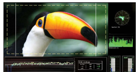
LKFS Audio Loudness Measurement - Digital Loudness Audio Metering with selected channel measurement in LKFS scale.
