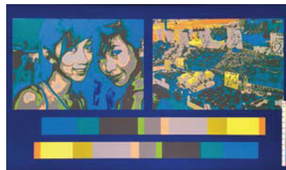
False color function refers to a group of color rendering methods used to display images in color which were recorded in the visible or non-visible parts of the electro-magnetic spectrum. A false-color image is an image that illustrates an object in colors that differ from those a photograph ( a true color image ) would show.
