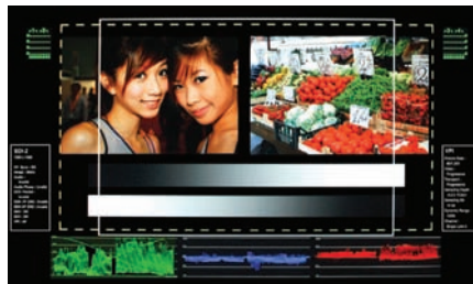
Advanced Waveform + VPID + Marker SDI-1, Waveform, (Y,Cr,Cb), 16 CH Audio Level Meter, VPID & Marker
